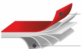
High Slip layer to prevent sticking of the external film layer on a pallet to the film on the pallet next to it
